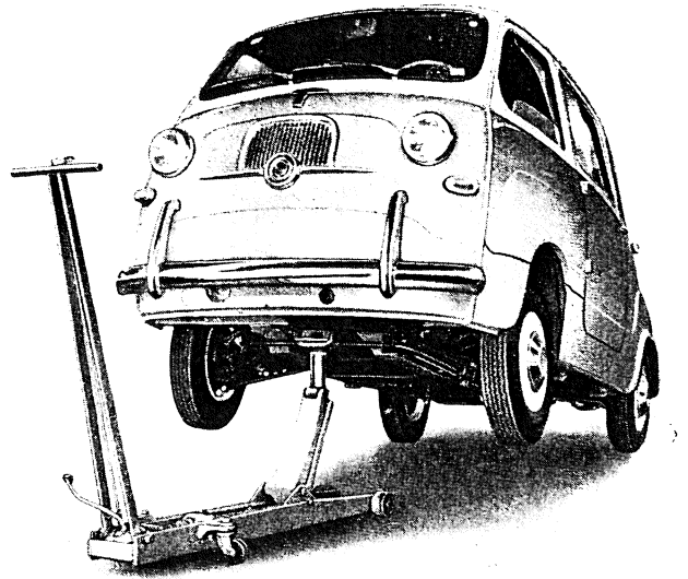
Fig. 9 - Raising Multipla front end with hydraulic jack Arr. 2027.
