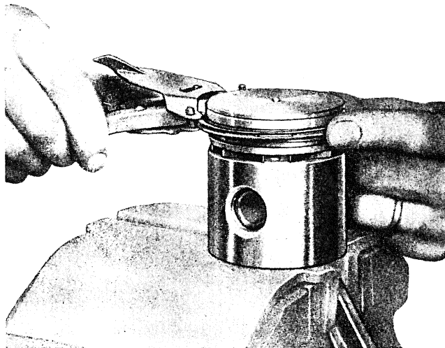
Fig. 43 - Fitting piston rings with installer A. 10114.
