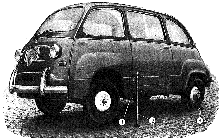
Fig. 378 - Jacking up the car.
